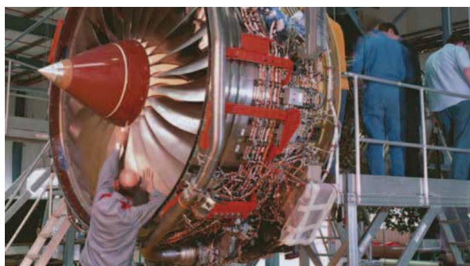
Flins Assembly line - Installation of an Airbus reactor © CCI Versailles-Yvelines
